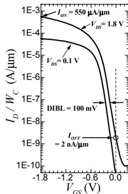
**Fig. 8.** Subthreshold and  $I_D$ - $V_{DS}$  characteristics for a representative  $L_G = 200$  nm VRG-pMOSFET with  $V_{DD} = 1.8$  V. These data are normalized to the coded width  $W_C$  (the device perimeter is  $\approx 2W_C$ ). With an  $I_{OFF} = 2$  nA/ $\mu\text{m}$  at  $V_{GS} = 0$  V and  $V_{DS} = 1.8$  V, the drive current is  $550$   $\mu\text{A}/\mu\text{m}$  at  $V_{GS} = V_{DS} = 1.8$  V.
