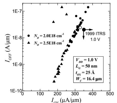
**Fig. 12.**  $I_{ON}$ - $I_{OFF}$  trend for a set of  $L_G \approx 50$  nm devices approaches the 1999 ITRS target for 1.0 V operation, even with a relatively thick 25 Å (TEM) gate oxide. The device of Fig. 11 is indicated by the open circle.
