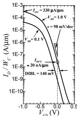
**Fig. 11.** Subthreshold and  $I_D$ - $V_{DS}$  characteristics for a representative  $L_G = 50$  nm VRG-pMOSFET with  $V_{DD} = 1.0$  V. With an  $I_{OFF}$  of about 20 nA/ $\mu\text{m}$ , this device drives 330  $\mu\text{A}/\mu\text{m}$ .
