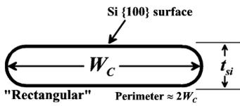
**Fig. 7.** Planview geometry of the VRG-MOSFET defining the coded width  $W_C$ .
