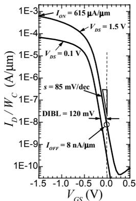
**Fig. 9.** Subthreshold and  $I_D$ - $V_{DS}$  characteristics for a representative  $L_G = 100$  nm VRG-pMOSFET with  $V_{DD} = 1.5$  V. This device has a 1.5 V roadmap target  $I_{OFF}$  of 8 nA/ $\mu\text{m}$  with a very high drive current of 615  $\mu\text{A}/\mu\text{m}$ .
